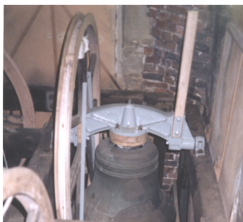
The 5th bell with new headstock, new stay and modified wheel.
